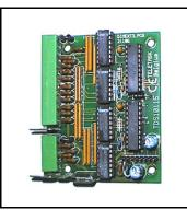
Optional dimmer board for MICROS with 16 analog outputs 0-10V
