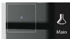
**Light, device, mood:** Any function that can be switch on/off, can be controlled on the AURUS-OLED. The icon as well as the indication LED will shine as the light, device or mood are switched on.
