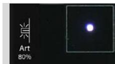
**Dimmer:** A dimmer can be controlled on a single button. By a SHORT push you can switch on/off the dimmer. By pressing LONG, you can dim up or down.
