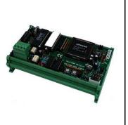
Interface to the AUDIOACCESS PX600 multiroom – multi source audio system. Permits the simultaneous use of up to 6 audio sources in up to 5 audio zones.
