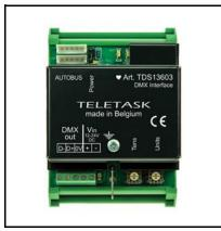
TheTDS13603 DMX interface can integrate up to 32 DMX compliant channels with the TELETASK domotics system (ex. 10 x DMX-RGB lighting unit + 2 independent DMX devices).
