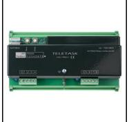
The TDS13501 relay interface to be connected to the AUTOBUS with 8 output contacts 10A/230V for general purpose ON/OFF or pulse control. The internal relays are plug-in type, for easy replacement.
