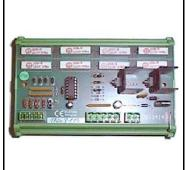
This booster module transforms up to four 0-10V analog outputs of a TELETASK central unit, to up to four 1-10V outputs to control HF fluorescent lamp electronic (dimmable) ballasts.
