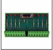
This module is 8 channels open collector output module.
