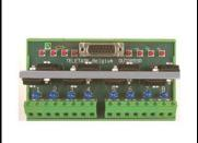
Relay module with 8 voltage free, solid state contacts, based on a high power triac with zero cross detection and switching. The module is to be connected to the TDS central unit by means of a dedicated cable (ref. TDS90101,TDS90103,TDS90105 or TDS90110). Each relay has its own ledindicator (when led active, the relay is active and the normal open contact is closed).
