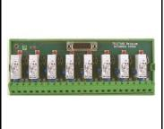
Relay module with 8 voltage free, change over, contacts. The module is to be connected to the TDS central unit by means of a dedicated cable (ref. TDS90101,TDS90103, TDS0105 or TDS90110). Each relay has its own ledindicator (when led active, the relay is active, the normal open contact is closed and the normal closed contact is open).
