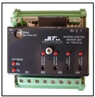
The TELETASK stand alone unit is a small control unit for a safe and independent access control system using the AUTOBUS cable and the TELETASK access control units (TDS12140 chipcard reader and TDS12142 proximity reader).
