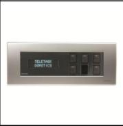
Touch panel with 5 buttons, for BTicino LIGHT and LIVING front plates, equipped with led's in every button, infra red receiver, IR-LINK output, buzzer and large VFD display (2 x 16 characters) for the read-out of different values (temperatures, humidity levels, light levels and messages. The 5 buttons are pre-programmed to be used for temperature control.
