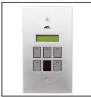
Touch panel TELETASK design, with 5 buttons with led indication in each button. Provided with IR-link output, buzzer and LCD-screen with back-lighting (2 x 16 characters). The display is to be used for displaying temperatures, humidity, light and messages and alarms. The 5 buttons are pre-programmed to be used for temperature control.
