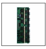
Relay extention board for the PROJECT central unit. By mounting one or up to two of these expantion cards, the standard nr. of 48 relays, can be extended from 48 to 2x48 or 3x48 outputs for OUT08x relay modules. If two extra boards are mounted the total relay outputs become 144 (without the relay interfaces which can be connected on AUTOBUS)
