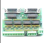
The dimmer-to-relay module transforms 16 dimmer outputs to 16 relay outputs.
