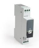
This 350 W universal power dimmer is intended for DIN-rail mounting and is 1 module wide. This power dimmer is suited for dimming traditional lights, electronic transformers and LED lights. The dimmer has a 0-10V input signal and 230V 50Hz power unit (leading or trailing edge dimmed; set by dip switched on the power dimmer itself).
