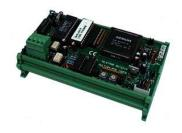
TELETASK Interface to connect a Honeywell GALAXY (type 8, 18, 60 or 500) or a GALAXY G3 or a GALAXY DIMENSION security system to the TELETASK system. This interface makes it possible to use the motion detectors of the Security system to control
